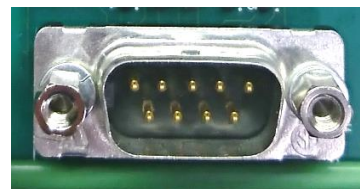
Figure 3. Male DE-9 Serial Connector Pinout
